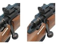
To engage the safety,pull the safety fully to the rear. when you are ready to fire,push the safety forward. 9.Adjust the hop-up.
